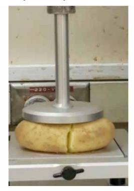
Figure 4. Force-deformation of food materials (ASAE, 2002).
