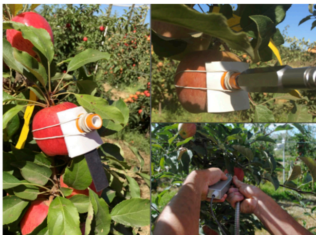
Figure 1. Details of the method developed to measure chlorophyll fluorescence parameters in apple fruit skin using a movable shutter clip under field conditions.
