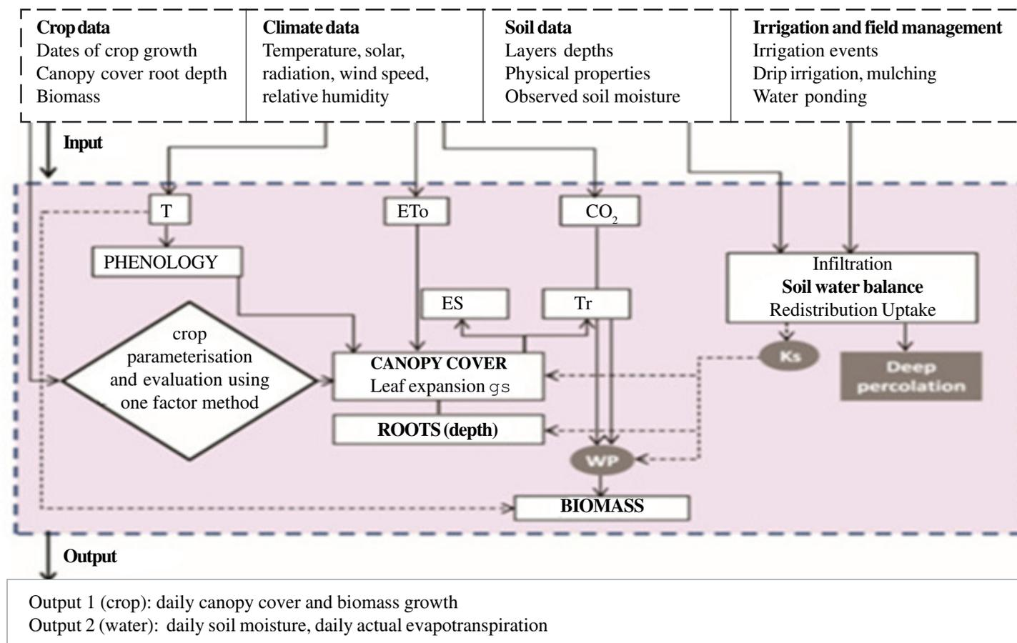
Figure 1. Flow chart for parameterisation of the AquaCrop adapted from Raes *et al.* (2009) and Steduto *et al.* (2009). T = temperature, ETo = potential evapotranspiration,  $g_s$  = stomatal conductance, WP = water productivity coefficient, Ks = stress coefficient, Es = soil temperature and Tr = crop transpiration.
