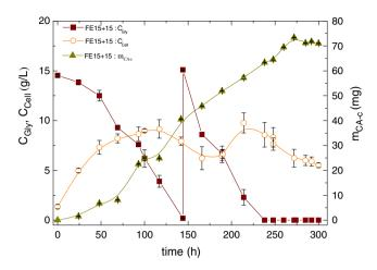
**Fig. 6.** Time courses of glycerol ( $C_{Gly}$ ) and cellular ( $C_{cell}$ ) concentrations, and cumulative CA mass ( $m_{CA-c}$ ), in the fermentation broth during extractive fermentation at 20°C with one glycerol pulse (EF15 + 15).
