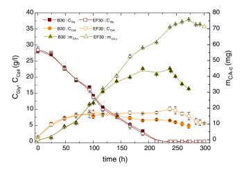
**Fig. 5.** Time courses of glycerol ( $C_{Gly}$ ) and cellular ( $C_{cell}$ ) concentrations, and cumulative CA mass ( $m_{CA-c}$ ), in the fermentation broth during conventional (B30) and extractive (EF30) fermentations at 20°C with 30 g/L initial glycerol concentration.
