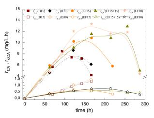
Fig. 7. Profiles of CA production rate ( $r_{CA}$ ) and CA degradation rate ( $r_{dCA}$ ) during conventional (B15 and B30) and extractive (EF15, EF30, and EF15 + 15) fermentations.
