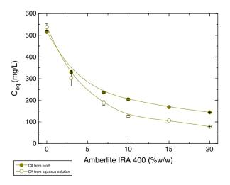
**Fig. 3.** CA concentrations at equilibrium ( $C_{CAe}$ ) as a function of the quantity of IRA 400 used: CA from broth and CA from aqueous solution.
