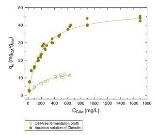
Fig. 2. Adsorption isotherms for the adsorption of CA on IRA 400 resin: Aqueous solution of Clavulin® and cell-free fermentation broth, at 25°C and pH 7.0.
