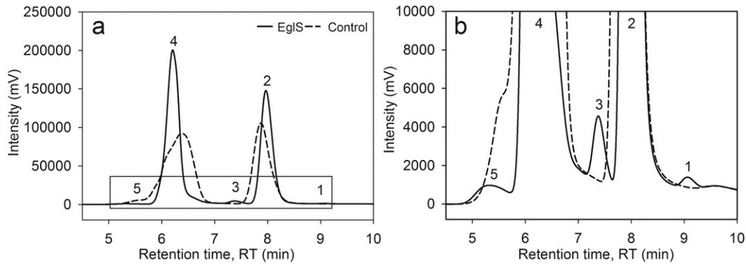
**Fig. 3.** HPLC chromatograms of sugar end products from the hydrolysis of CMC (1% w/v) by recombinant endoglucanase (EglS) and control in 50 mM sodium citrate buffer (pH 4.8) at 50°C for 30 min, peak 1: glucose, 2: sodium citrate, 3: cellobiose, and 4–5: gluco-oligomers of CMC. The rectangular area in chromatogram (a) is enlarged in (b).
