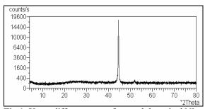
**Fig 1**: X-ray diffractogram of normal deposited Ni thin film (sample NiO)
