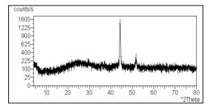
**Fig 2**: X-ray diffractogram of helical deposited Ni thin film (sample Ni40)
