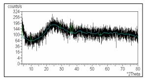
**Fig 3**: X-ray diffractogram of zigzag deposited Ni thin film (sample Ni70)
