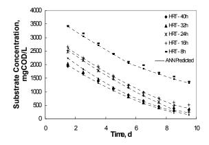
Fig. 3 Experimental and ANN Predicted COD Vs Time – Initial Substrate Concentration of 4475 mg COD/L
