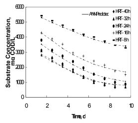
Fig. 4 Experimental and ANN Predicted COD Vs Time – Initial Substrate Concentration of 6730 mg COD/L
