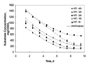
Fig. 2 Experimental and ANN Predicted COD Vs Time – Initial Substrate Concentration of 2250 mg COD/L
