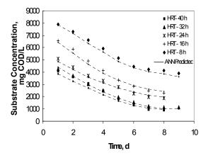
Fig. 5 Experimental and ANN Predicted COD Vs Time – Initial Substrate Concentration of 8910 mg COD/L
