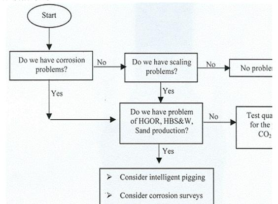
Fig 9. Surveillance for Corrosion and Scaling
