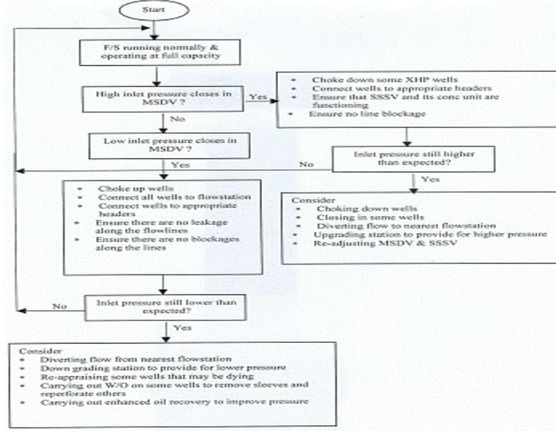
Fig 5. Flow chart for pressure surveillance
