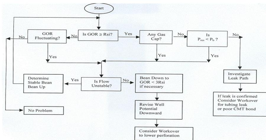
Fig 2. Flow chart for well producing at high HGOR
