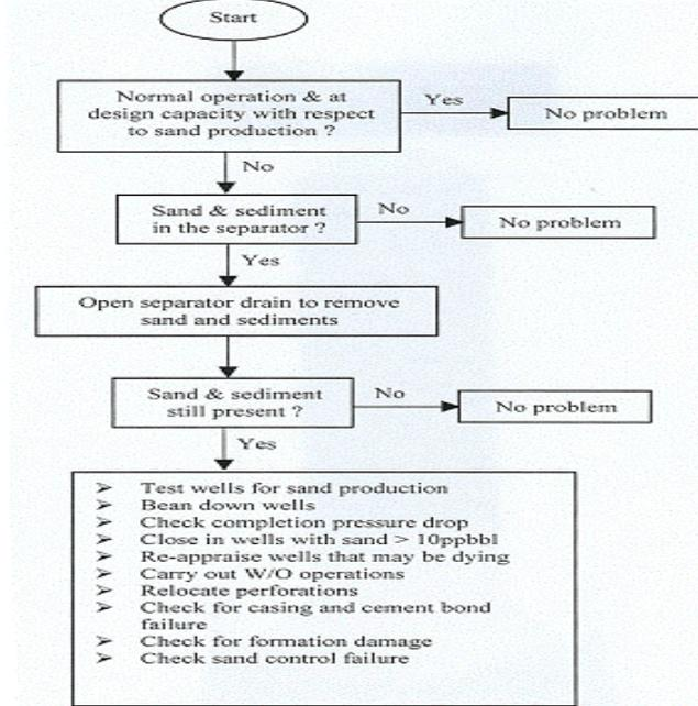
Fig 7. Surveillance for sand production from flow stations
