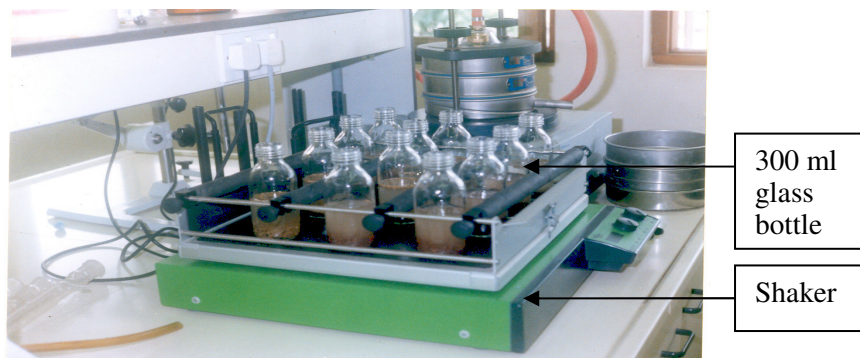
Plate1: Phosphorus sorption experiments in a slow rotating shaker
