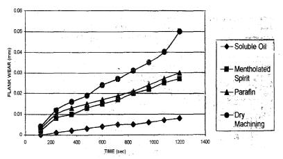
Fig. 8: Graph of flank wear (mm) against time (sec) with carried tipped tool and medium carbon steel
