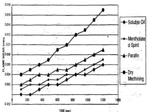
Fig. 7: Graph of flank wear (mm) against time (sec) with carbide tipped tool and mild steel workpiece
