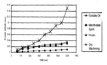
**Fig. 4:** Graph of flank wear (mm) against time (sec) with high speed steel cutting tool and medium carbon steel
