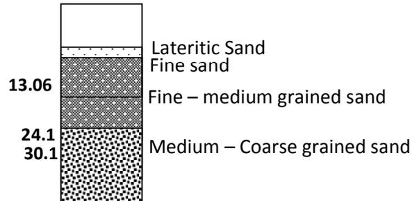
Fig 4: Borehole lithologic log at Ejeme – Aniogor.
