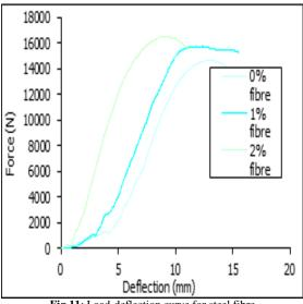
Fig 11: Load-deflection curve for steel fibre
