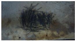
Fig 3: Steel fibres
