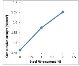
Fig 10: Influence of steel fibre content on compressive strength
