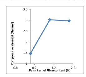
Fig 8: Compressive Strength (MPa) against Palm kernel fibre content (%)
