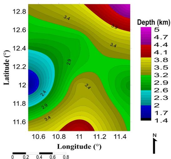
**Fig. 7** Depth to the top ( $Z_t$ ) of magnetic sources contour map (Sedimentary thickness). (Contour interval of 0.1km)
