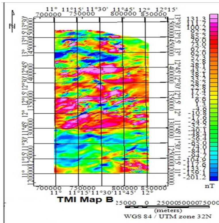
Fig.3. Total Magnetic Intensity (TMI) Map B (Second set of obtained aeromagnetic map).
