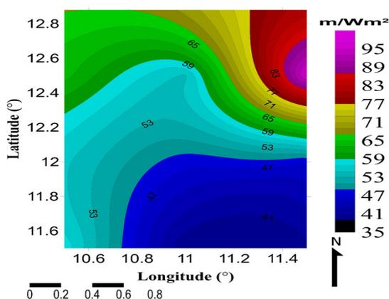
Fig. 10. Surface heat flow map of the study area (Contour interval of  $2m/Wm^2$ ).
