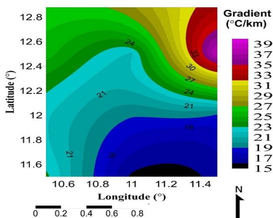
Fig. 9. Geothermal gradient contour map of the study area (CI -  $1^{\circ}C/km$ )
