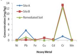
Fig. 2: Mean Concentration (mg/kg) of Heavy Metal in Site A, Site B and Remedial soil from Dareta
