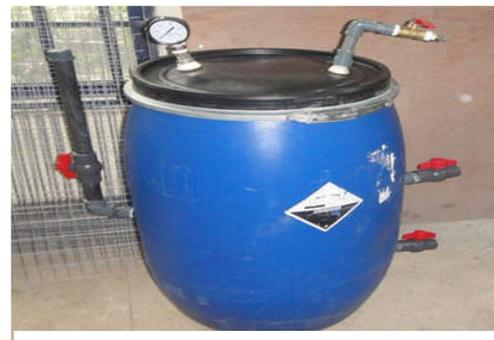
Fig 2: Biogas digester reactor Substrate Preparation:
