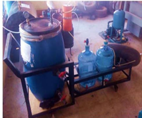
**Fig 5:** Biogas production and purification system
