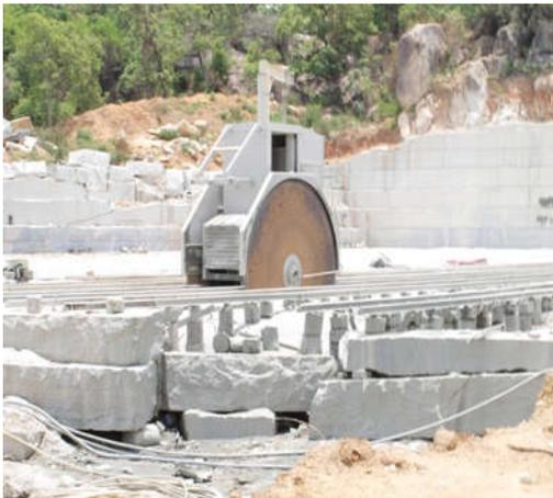
Fig 5. China dimension stone cutting equipment at Kporokpo village in Lokoja area, Nigeria
