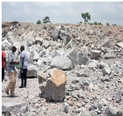
Fig 2. Field photograph of biotite granite blasted for production of aggregates at Kporokpo village.
