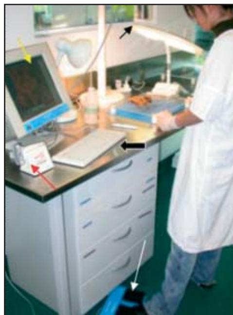
Figure 1: The Milestone MacroPath system comprising a camera (black arrow), foot pedal control with zoom in, zoom out and freeze pedals (white arrow), formalin-resistant touch screen monitor with attached splash-proof computer (yellow arrow), infra-red bar code scanner (red arrow) and keyboard (broad arrow)
