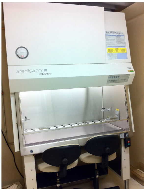
Figure 1: Biological security cabinet. It is a special cabinet with constant airflow from the back to the front and from the bottom to the top, which permit working with highly virulent organisms such as M. tuberculosis . In this equipment, mice are infected with virulent microbacteria and are euthanised for organ harvesting for microbiological, immunological, and histopathological evaluations. The biological security cabinet is a part of biosafety level-3 (BSL-3) facilities of the animal house in the National Institute of Medical Sciences, Mexico City.
