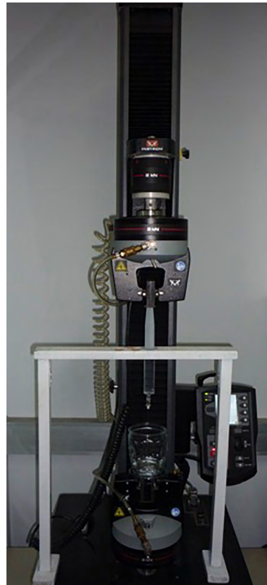
Figure 1. The Instron 5940 device is a single column tabletop model testing system to measure the initial and the maintenance force of the syringe and needle pairs
