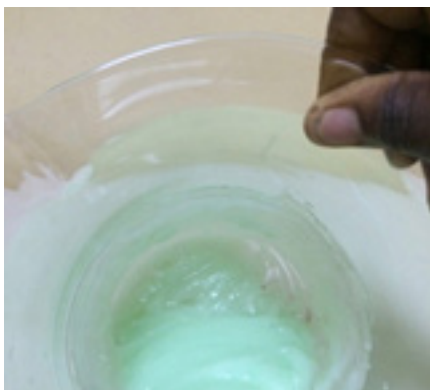
Figure 1: Beaker with the fortified gel made from plain gel, 0.5% chlorhexidine and 70% ethyl alcohol in a 20:2:1 composition (note the opaque pale green colour)
