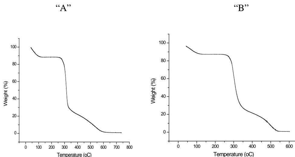
**Figure 5: TG thermogram of native (A) and acetylated (B) acha starches**
