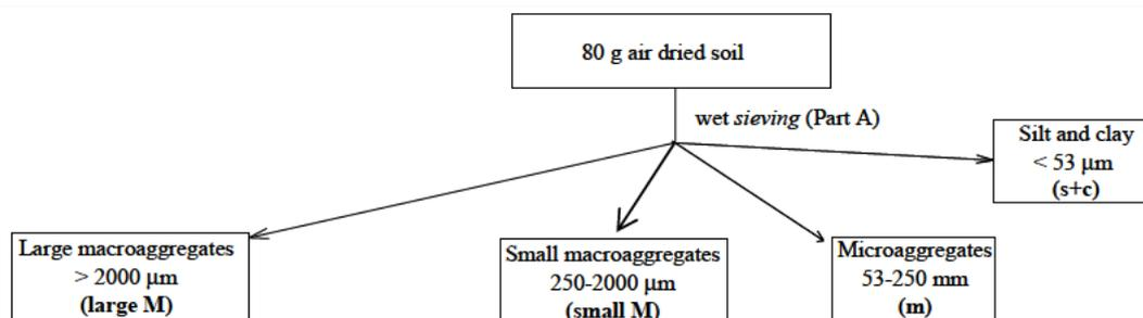
**Figure 1: Procedure for Soil Organic Carbon Fractionation as adopted from Six (2011)**
