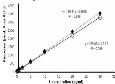
**Fig 1:** Standard calibration curve (mean peak area vs. concentration in  $\mu\text{g/ml}$ ) for metronidazole dissolved in mobile phase ( $\blacklozenge$ ) and extracted from plasma ( $\circ$ )
