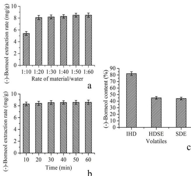
**Figure 2:** Optimal conditions of hydrodistillation; (a) optimization of ratio of material/water; (b) optimization of distillation time; (c) comparison of (–)-borneol content of volatiles for three methods
