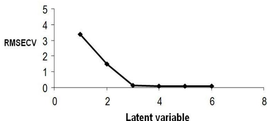
**Figure 3:** RMSECV plots for the cross validation results of the training set as a function of the number of factors used to construct the calibration models**Table 2:** Determination of CHP and DX in validation set by the proposed multivariate calibration methods
