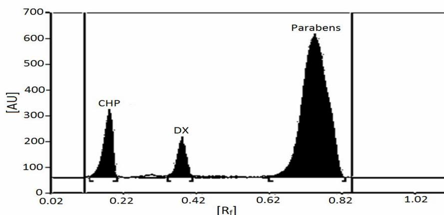
**Figure 4:** Thin layer chromatogram of CHP, DX and Parabens (MP and PP) using developing system, chloroform: methanol (93:7 v/v)
