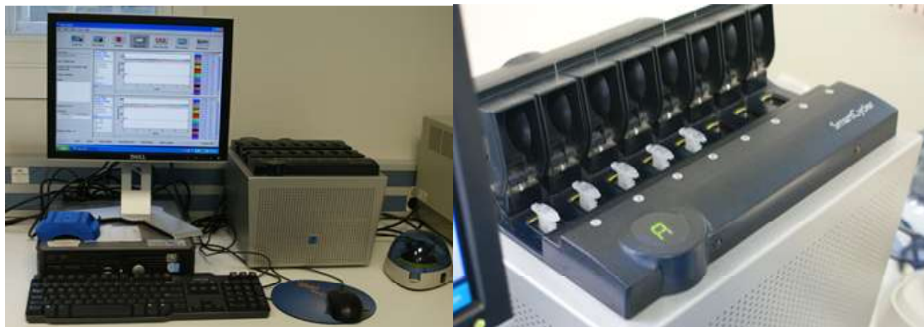
Figure 1. Smart Cycler equipment, where DNA amplification is performed and the results are analyzed
