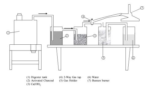
Fig. 2: Schematic diagram of the anaerobic digestion experiment
