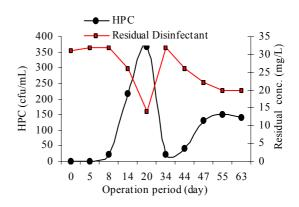
Fig. 4: Variations of HPC in different residual Nanosil concentrations during the experiment (Outdoor Swimming pool)
