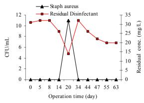
Fig. 6: Variations of *Staphylococcus aureus* in different residual Nanosil concentrations during the experiment (Outdoor Swimming pool)
