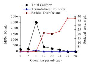
Fig. 2: Variations of total coliform and thermotolerant coliform in different residual Nanosil concentrations during the experiment (Indoor Swimming pool)
