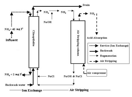
Fig. 1: Schematic diagram of designed pilot
