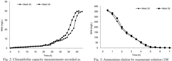
rig. 2: Chinoptilolite capacity measurements recorded as mg of  $NH_4^{+/g}$  of dry clinoptilolite in continuous system
