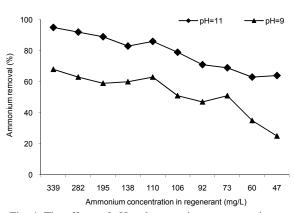
Fig. 4: The effects of pH and ammonium concentration on removal efficiency of ammonium by air stripping
