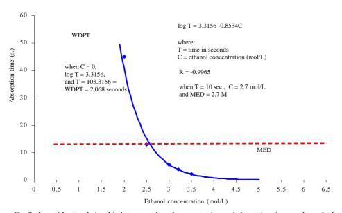
Fig. 2: Logarithmic relationship between ethanol concentration and absorption time used to calculate water repellency severity and persistence
