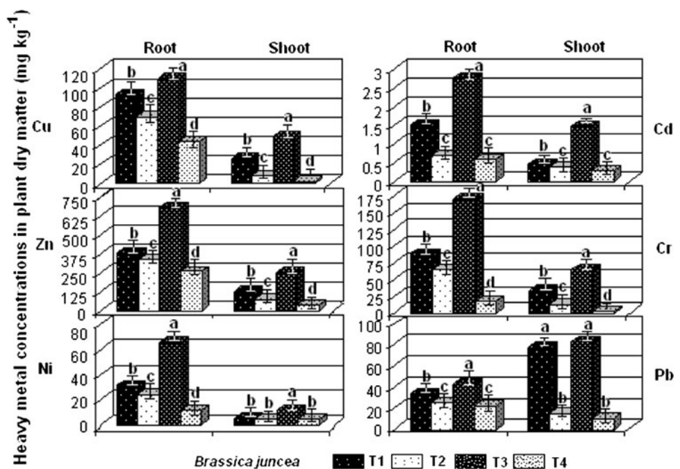
Fig. 2 Heavy metal concentrations (mg kg -1 dw) of B. juncea at different treatments (T1: sulfur, T2: gypsum, T3: EDTA, T4: control treatments) (Vertical bars indicate standard deviation, n = 4)
