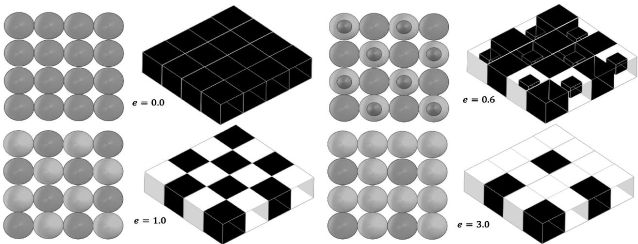
**Fig. 2** Effective bearing area as a function of packing state
