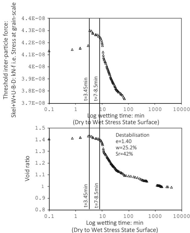
**Fig. 6** Timed variation of cohesive inter-particle forces (balanced destabilising inter-particle forces) upon wetting
