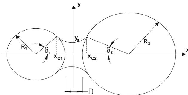
Fig. 3 Liquid bridge geometry between pair of quartz spheres
