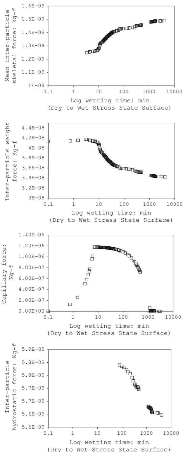
**Fig. 4** Variation of inter-particle forces on the dry-to-wet stress-state surface
