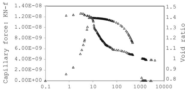
**Fig. 5** Timed variation of water tension and void ratio upon wetting
