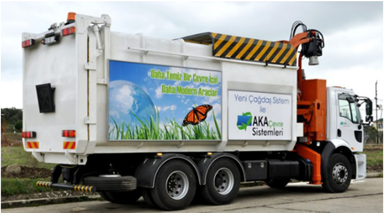
Fig. 4 Solid waste collection vehicle with robotic arm
