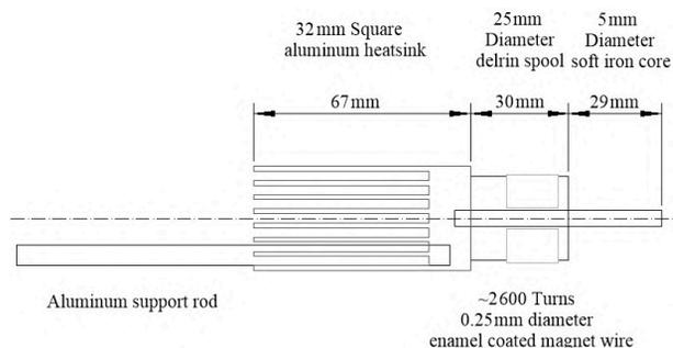
**Figure 2 Schematic illustration of the electromagnetic device**
