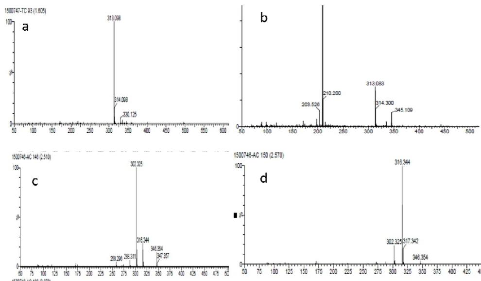
**Figure 5:** Mass spectra of aflatoxin B<sub>1</sub> in standard (a); *T. cordifolia*(b); *A. calamus* (c); *M. fragrans*(d)
